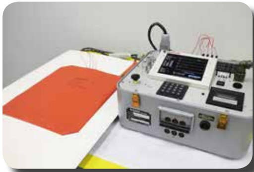
Smart Susceptor Heat Blanket connected to HCS9400-02 Smart Susceptor Hot Bonder in preparation for a composite repair.
