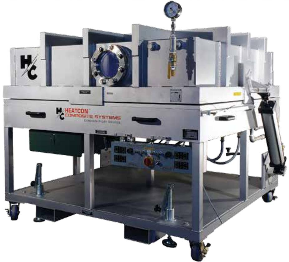
The HCS7600 series DVD Chamber is a custom designed, double vacuum, debulking chamber used for pre-curing composite repair patches resulting in a near-autoclave quality repair. DVD Chamber operation is an operator and/or repair-specific combination of traditional Hot Bonder controlled heat and bag-vacuum with operator controlled chamber vacuum.
