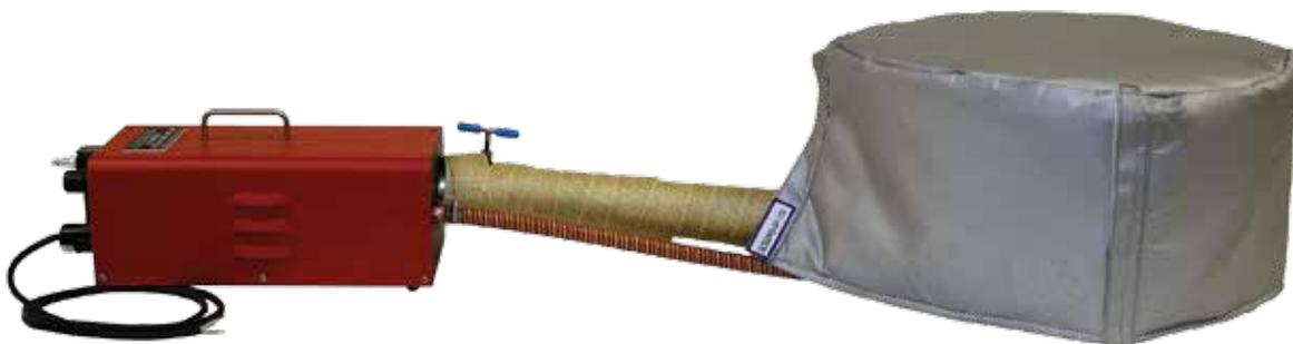
This Portable Hot Air Composite Curing System fills an important gap in composite repair techniques by applying heat to difficult shapes or hard to reach areas. Primary applications are composite repairs, secondary bonding, and modifications to composite structures. Powered and controlled by a Hot Bonder, it provides even heating of contoured surfaces and can be effectively used in place of standard silicone rubber heat blankets.
